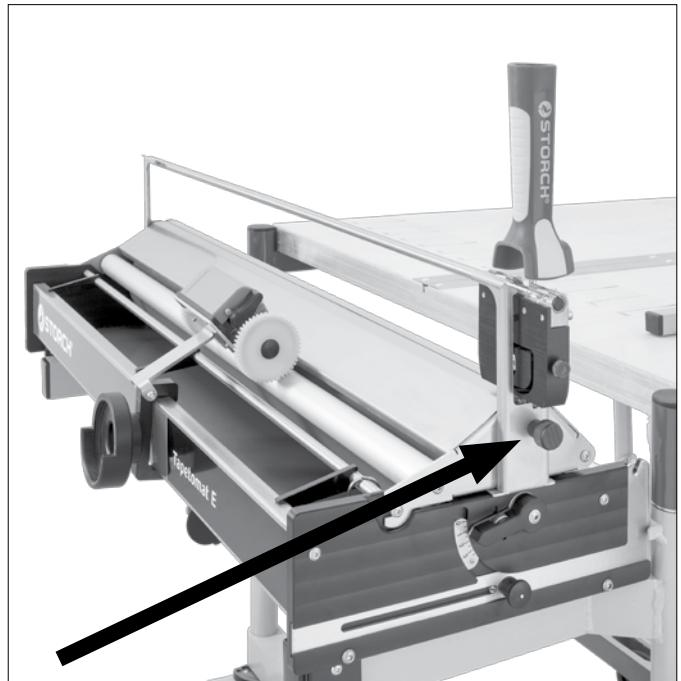
Secure the fastening nuts on the inside of the hood with the black screws, align the cutting cart and tighten the screws.
