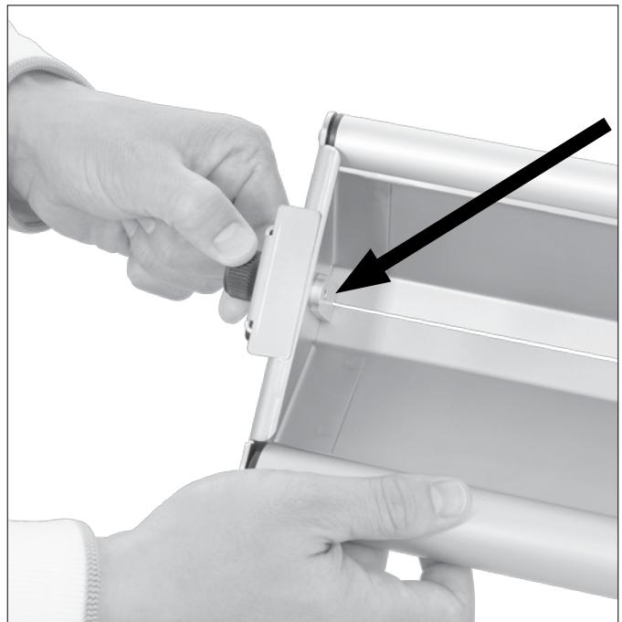
Insert the rotary cutter into the cutting cart's clamp, applying pressure. Next, tighten the clamp with the side screw and move the bolt on the handle downwards.
