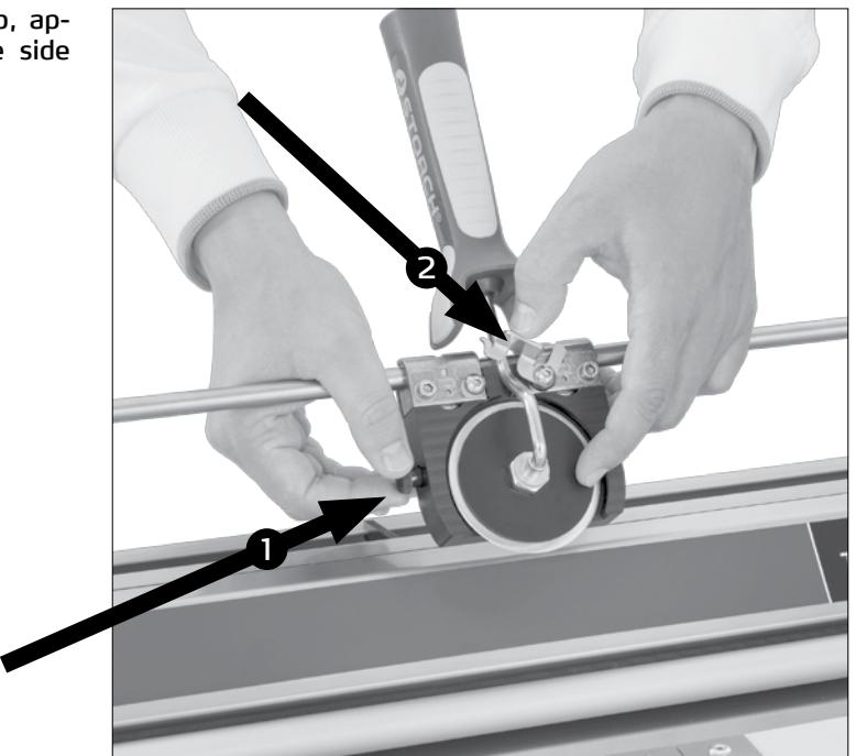
Guide the cart along with rotary cutter into the middle of the frame, gently pull upwards and insert the cutter into the cutting slot.
